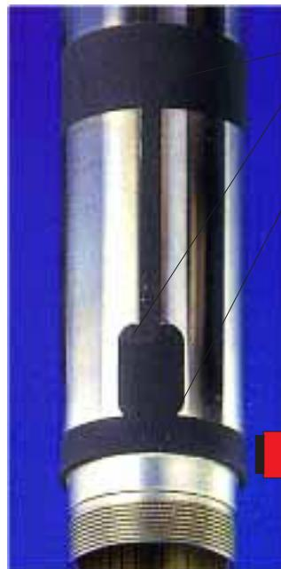
Strain gage encapsulated
