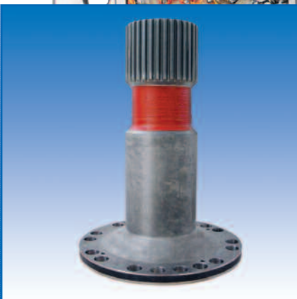
Torque measurement on the main rotor mast of helicopters
